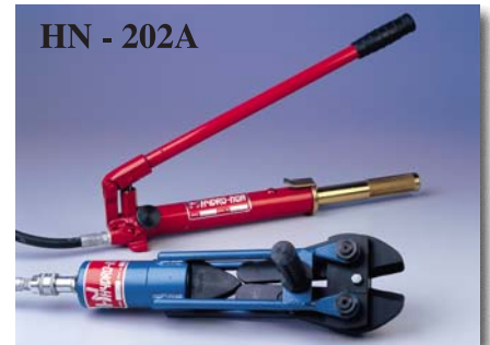
HN - 202A Hand Pump: 3.6 kg Cutter: 7.85 kg Cutting: Tempered Steel: 16 mm Standard: 20 mm Dim(Lxwxh):425x125x170 mm Max. Power:35,000 kg.
