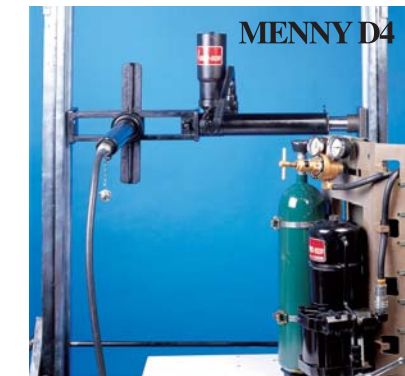
MENNY D4 Hydraulic Pump: 21.35 kg Door Buster: 21.98 kg Width (closed): 732 mm Width (open): 980 mm Extensions: (up to 1350 mm)
