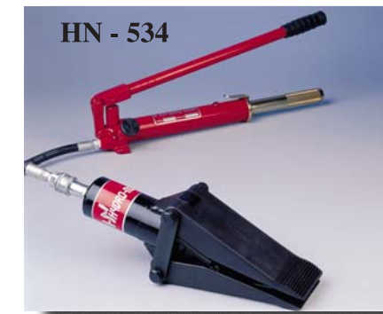
HN - 534 Spreader: 9.36 kg Hand Pump: 3.6 kg Dim(Lxwxh):345x125x110 mm Closed: 5 mm Max. Open Spread: 115 mm Max. Power: 7500 kg
