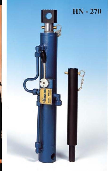
Weight: 14.2 kg Opening Power: 9,812 kg Pulling Power: 4144 kg Working Pressure:500 bar Length (closed): 600 mm (open): 953 mm (without extension), 1263 mm (with extension HN-271) 1653 mm
