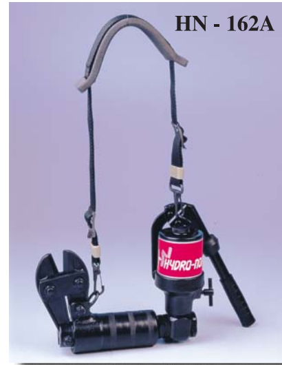
HN - 162A Weight: 4.6 kg Dim(Lxwxh):245x102x190 mm Cutting: Tempered Steel: 7 mm Standard: 13 mm Cutting Power: 13,800 kg.
